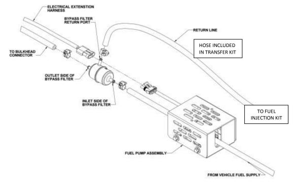
Figure 3. Fuel Pump and Filter Detail
