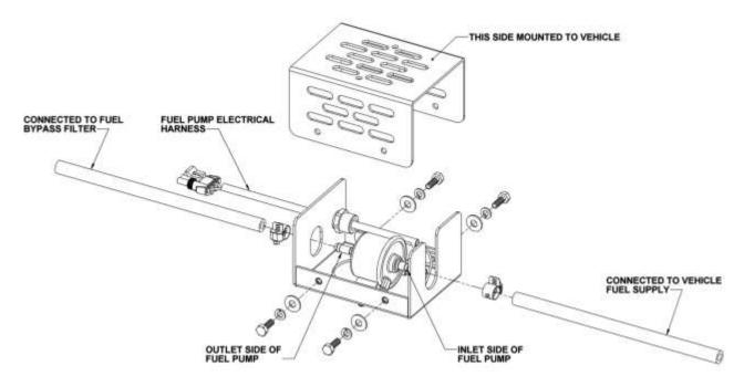
Figure 2. Fuel Pump Assembly Detail
