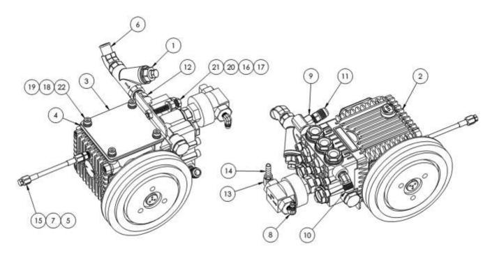
69-455, ASSY, WATER PUMP (GENERAL PUMP – FOR SERIAL #'S 757 AND UP)
