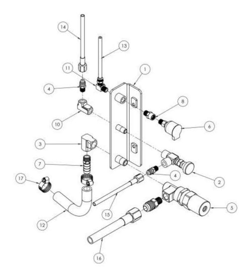
69-187 ASSEMBLY, BRACKET, MOUNTING, LOWER RIGHT
