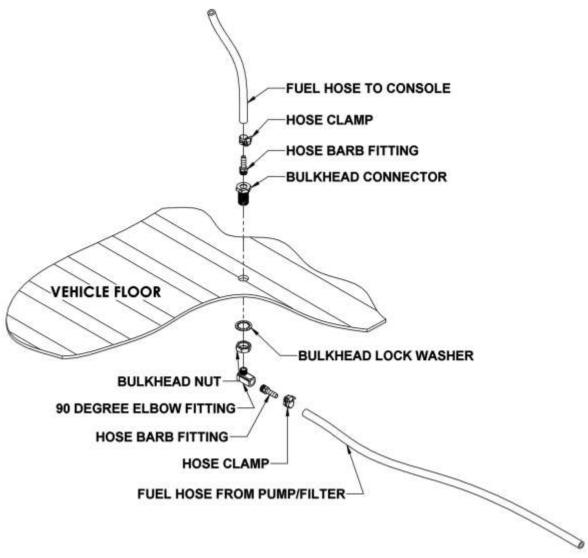
Figure 1. Fuel Line Bulkhead Assembly
