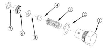
23-063 VLV, CHECK, CHECK VLV MANIFOLD
