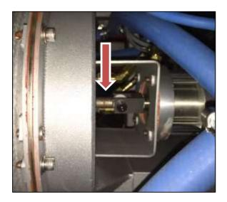
Every **100 hours**, remove the white vacuum tubes from the Bimba cylinder and add a 5-second shot of WD40 to each side of the cylinder. If the cylinder does not move freely, remove the cylinder by removing the four bolts at the front of the cylinder and take the cylinder apart. Clean the interior parts with a scotch-brite pad. Lube with WD40 and re-assemble the cylinder.
