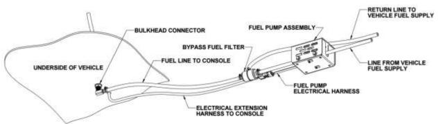
Figure 4. Vehicle Underside Fuel Line Installation
